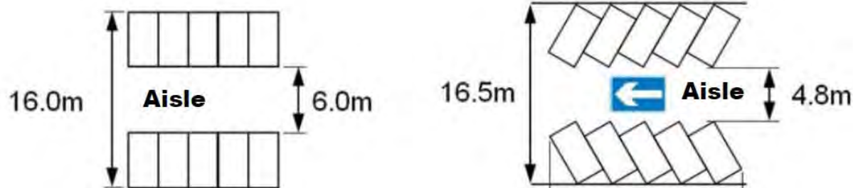
Figure 33.21: Accessory Building and Main Building Examples of Parking Aisle
